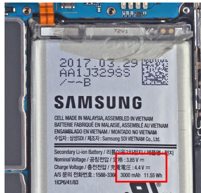
3.85 \text{ V} \times 3 \text{ Ah} \times 3600 \text{ s/h} = 41.6 \text{ kJ} .
