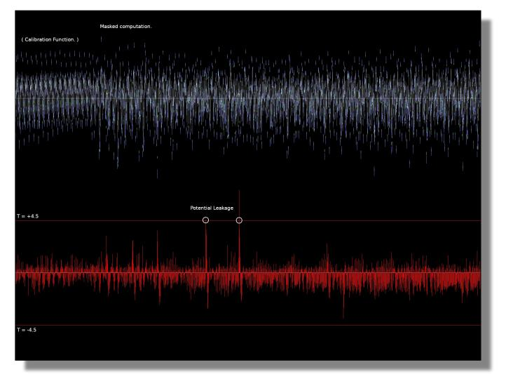
→ We use FPGA to emulate leakage of hardware post-quantum crypto modules. Try to apply ISO 17825.
