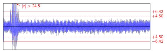
Zoom of the first PRF in a non-accelerated TVLA shows strong leakage.
